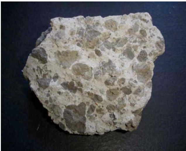
Figure 1 Chunk of Flowable Fill made from Insitu Clay Soil
