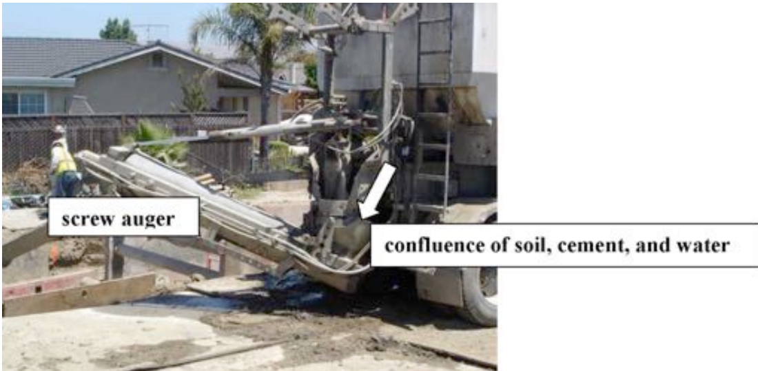
Figure 3 Mixing and Screw Auger on Volumetric Mixer
