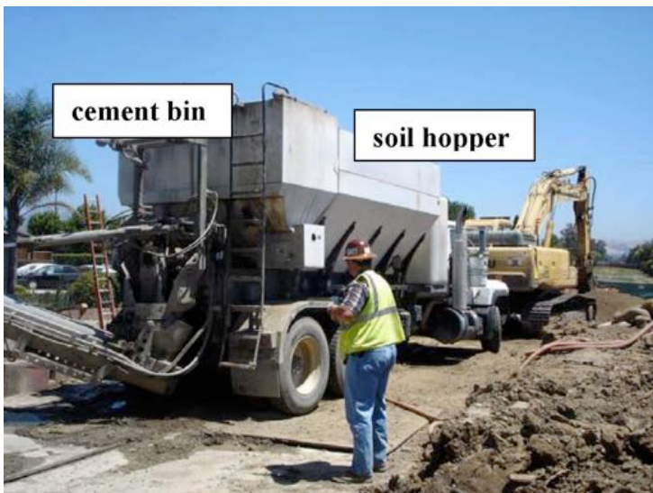
Figure 2 Volumetric Concrete Mixer used for Flowable Fill
